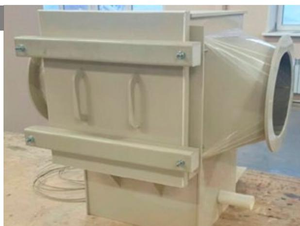
Also our company can make lining of electroplating baths with fluoroplastic materials. Casing lining of electroplating baths protects the bath sides from the impact of chemical solutions.
